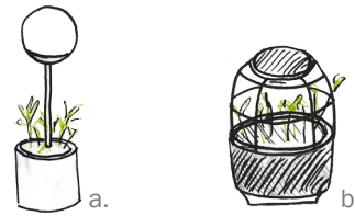
III.72: Structural principle: a. structural pole in the middle, b. grid formation
