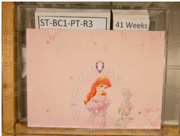
Fig. 2. Left: Sample with aerated cellular concrete and wallpaper. No growth is seen even after 41 weeks at 20 °C and 90 % RH. Right: Sample with gypsum board and wallpaper 4 weeks after adding 100 ml sterile water (rotated left 90°). The black growth is Chaetomium .
