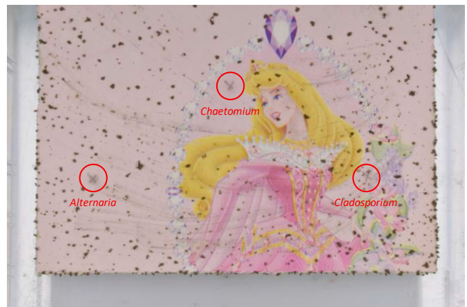
Fig. 2. Left: Sample with aerated cellular concrete and wallpaper. No growth is seen even after 41 weeks at 20 °C and 90 % RH. Right: Sample with gypsum board and wallpaper 4 weeks after adding 100 ml sterile water (rotated left 90°). The black growth is Chaetomium .
