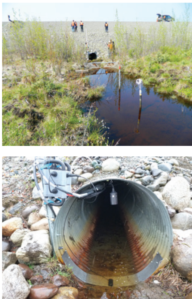
Figure 10.29 Instrumented culvert at the Beaver Creek experimental site, Alaska Highway, Yukon, Canada (sources: P  rier et al., 2014, and P  rier, 2015).
