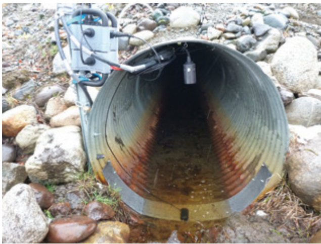
Figure 10.29 Instrumented culvert at the Beaver Creek experimental site, Alaska Highway, Yukon, Canada (sources: P erier et al., 2014, and P erier, 2015).
