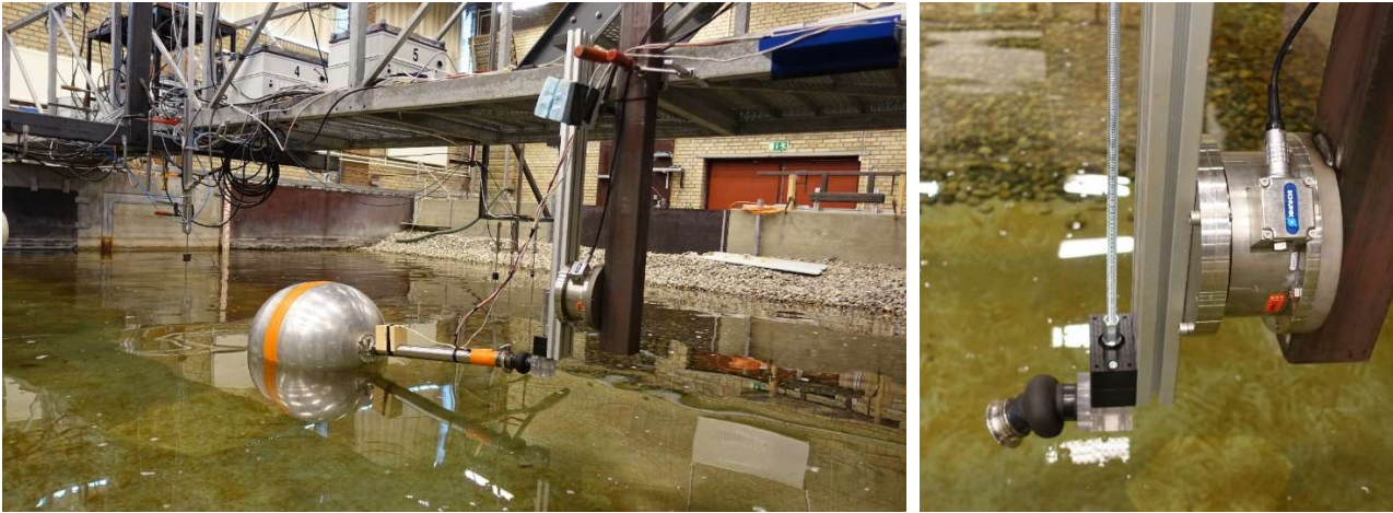
Figure 1: Setup in wave basin. Right photo shows the 6-axis force sensor and the mount.
