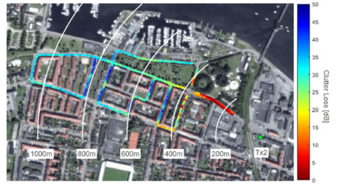
Fig. 3. Clutter loss measured at 18 GHz for the base station location Tx2 in Aalborg.
