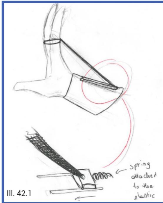
The concept is based on the sketch above (Ill. 42.1): a spring on the wrist area gives resistance to all the fingers through 3 guides on each.
