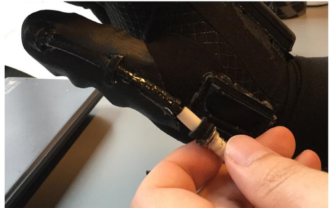
Ill. 62.4 *The spring unit is screwed to the rod*
