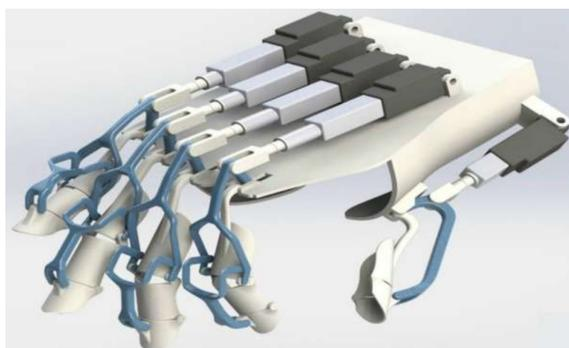
Ill. 42.2 Shells attached on top of the fingers interconnected with pistons (linear actuators) top support the hand movement to aid in rehabilitation.
