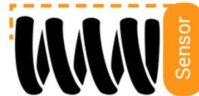
III. 54.4 Sensor on the side of the spring measuring the distance to the other end of the spring.
