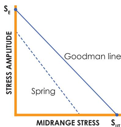
Shot Peening can be used to improve the life-time of a spring, it can improve the torsional fatigue strength by 20% or more. The size of the shot is about 0,40 mm which means the springs need to be designed to be able to be completely covered of the spring surface by the shots in order to make the method effective.
