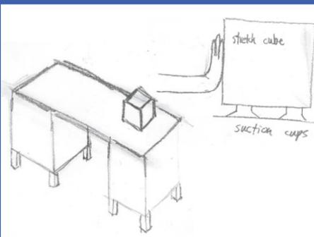
III. 41.2 The stretch-cube has suction cups on the bottom to make a stationary surface for stretching the wrist.
