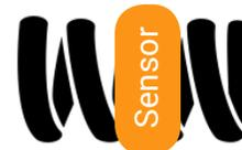
III. 54.5 Sensor on the spring itself measuring the distance between coils.
