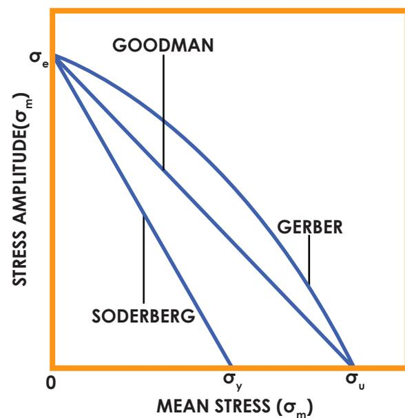
To find out when a spring will fail, it is held up against failure criterions: Gerber, Goodman and Soderberg, where Soderberg is the most conservative, and Goodman the least when using the Zimmerli data. The result is a factor of safety where numbers above 1 theoretically have infinite life and the bigger the number the more safety there is for the spring to hold.
