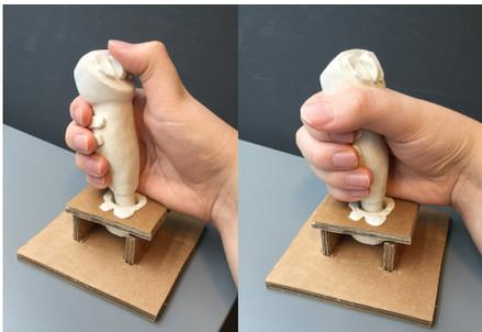
III. 27.1 The joystick is intended to give an ergonomic grip and have the buttons placed in an easy to reach position for the thumb, index and middle finger.
