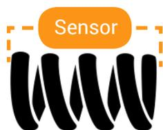
III. 54.2 Sensor on the side of the spring measuring the distance between the ends of the spring.
