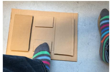
III. 27.3 The board on the left houses the buttons while the 'slipper' is used to move the mouse pointer.
