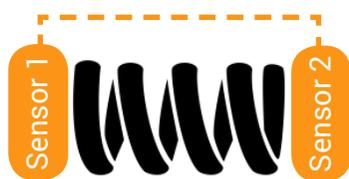
III. 54.2 Two sensors attached to the ends of the spring and measuring the distance between each others.
