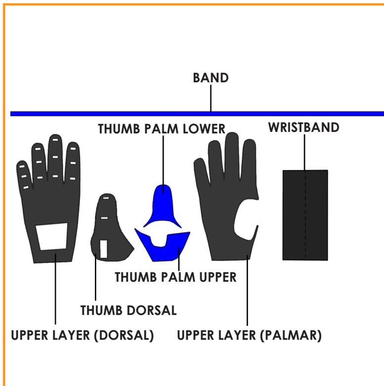
III. 71.3 Construction of the upper layer of glove
