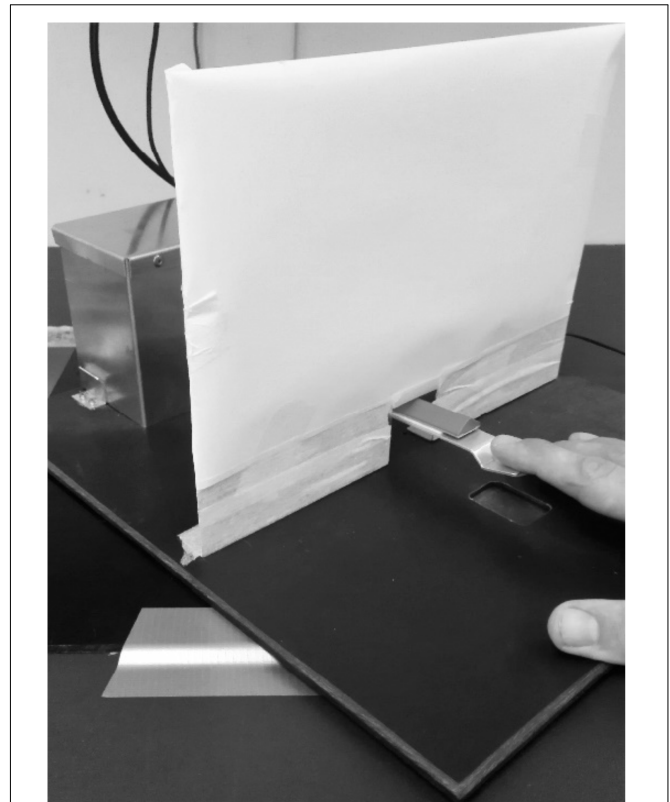
FIGURE 2 | Illustration of the custom-built passive tapping machine.
