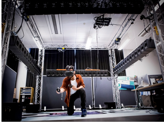
Figure 2. A 64-channel Wavefield Synthesis setup and Virtual Reality equipment at the Multisensory Experience Lab at Aalborg University Copenhagen.
