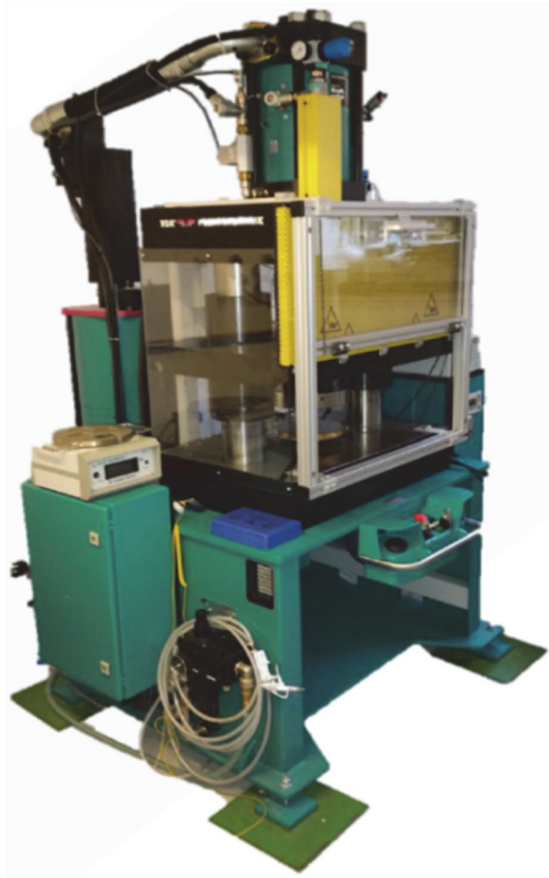
Figure 25. The 100 ton TOX air-driven press used for sample fabrication.
