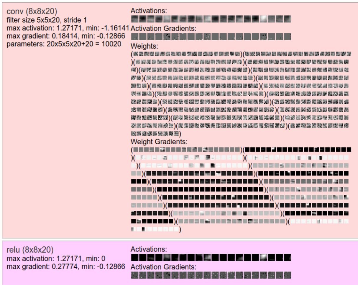
Figure 2.21: An example of the filters learned by the third convolutional layer of a neural network, trained on the CIFAR-10 dataset and ran through the visualisational demo of Stanford University at [36]. The input image is the same ship as on Figure 2.20
