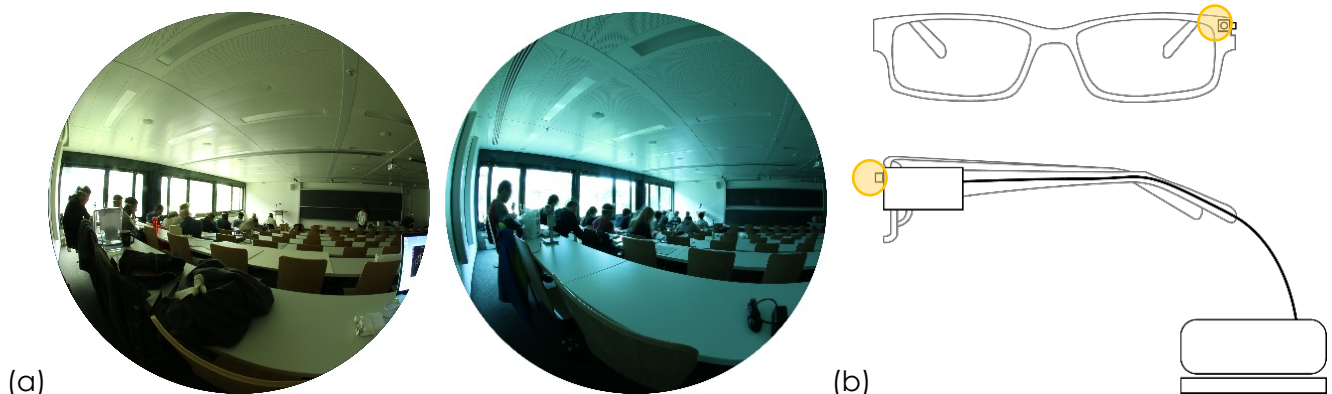
Figure 1. (a) Experimental design. Control group experienced daylight neutral conditions (left) and intervention group experienced red-impooverished daylight (right). (b) SMEAS, customized wearable device to measure vertical illuminance and irradiance.
