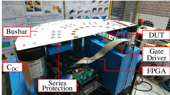
Fig. 2. Picture of NDT setup in the laboratory.
