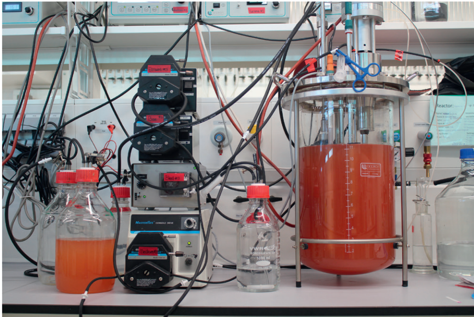
Figure 5.3 Anammox reactor with red granules containing Kuenenia stuttgartiensis . Image courtesy of Boran Kartal.
