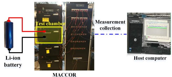
Fig. 8. The structure of the test bench
