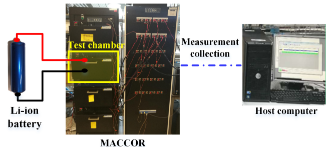
Fig. 8. The structure of the test bench
