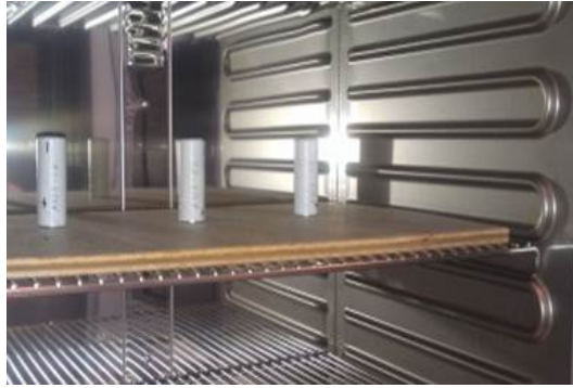
Figure 5.4: LFP/C battery cells stored in oven during one of the accelerated calendar lifetime tests.
