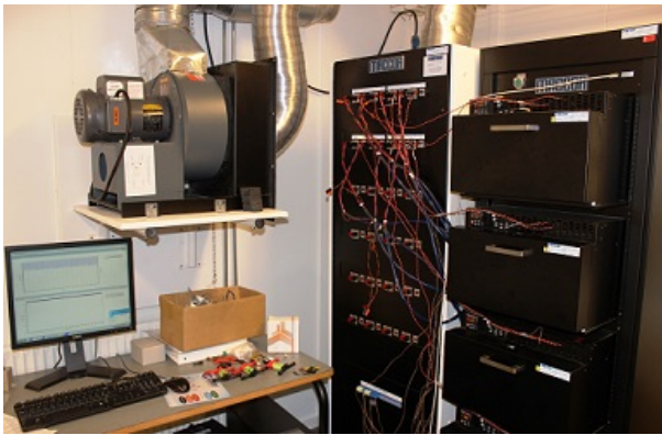
Figure B.2: Maccor battery test station.
