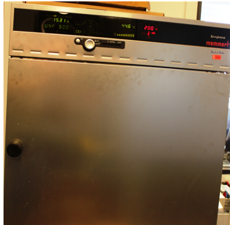
Figure B.3: Memmert UNP 500 universal oven used for accelerated calendar ageing tests.
