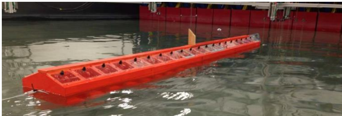
Figure 2. The 3-meter experimental model of the KNSwing.
