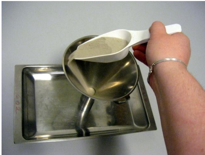
Figure 2: Material is filled in a small cylinder by carefully letting it slide down along the rim of the funnel.
