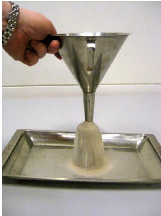
Figure 3: Small cylinder filled with material, and excess material running over.
