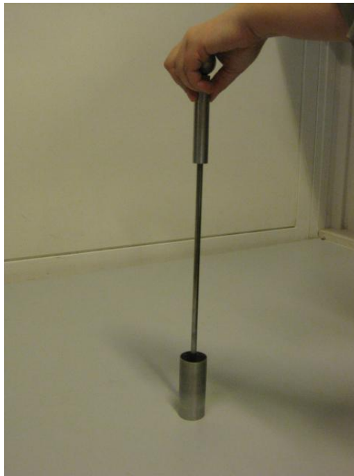
Figure 7: The drop weight is taken up to the stop block in the tamping.
