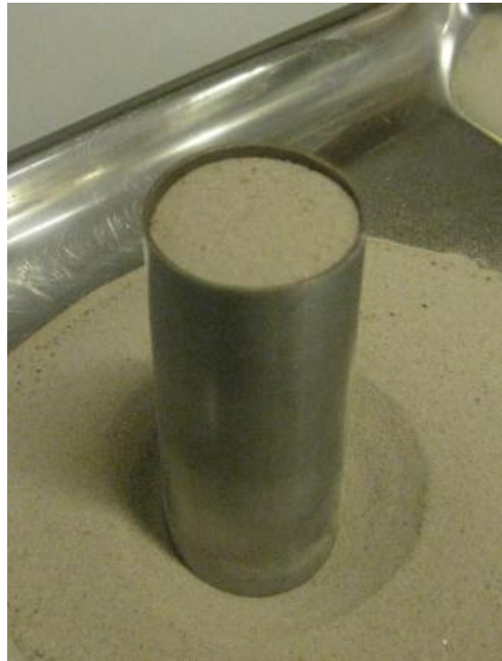
Figure 5: Levelled cylinder, before and after hard knocks in the table.
