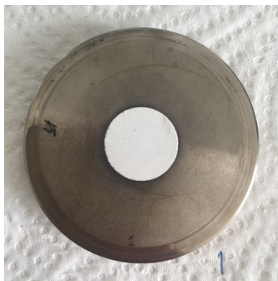
Figure 6 Tablet prepared for XRD analysis
