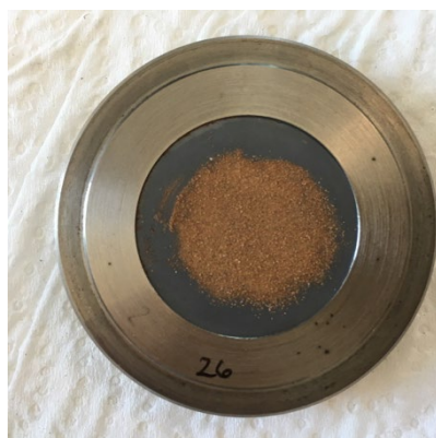
Figure 7 Powder sample prepared for XRD
