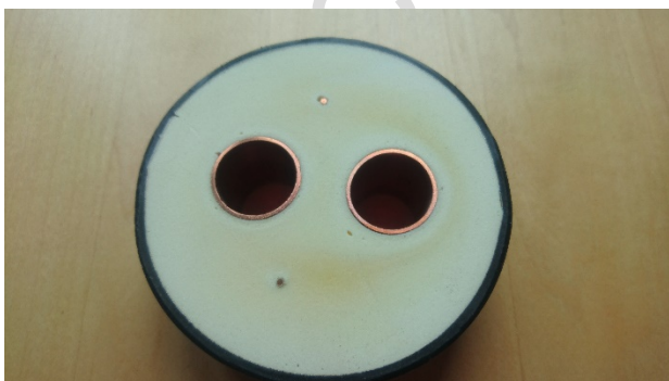
Figure 4: Double DH pipe system by Logstor.
