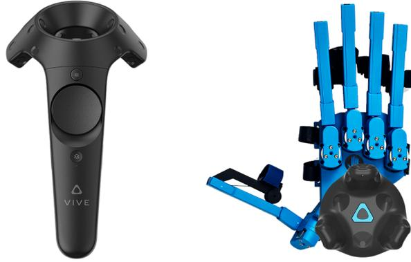
Figure 14.: Vive Controller (left) and SenseGlove (right) with a Vive Tracker.
