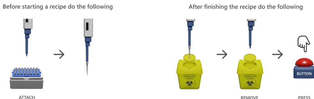
Figure 31.: Instructions displayed on the whiteboard. On the left instructions are given on how to begin a recipe. The user has to put on a tip (one tip is used per recipe). Upon finishing the recipe the user must discard the tip and press the red button to continue.
