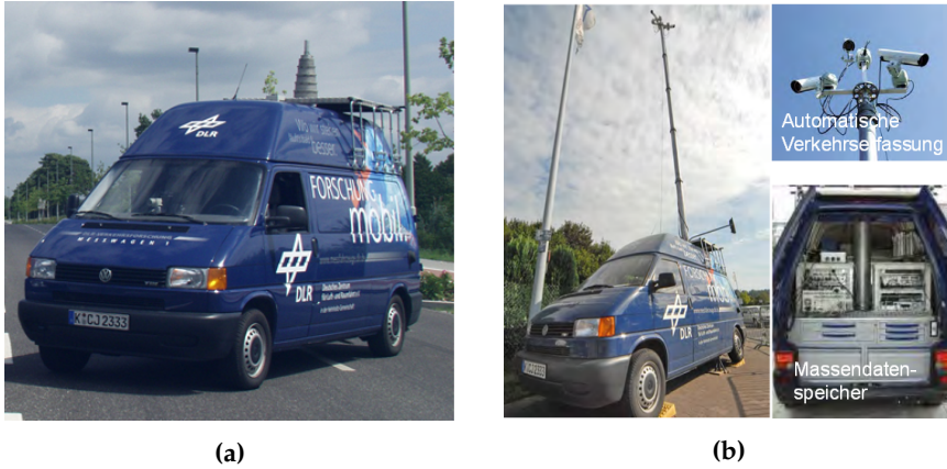
Fig. B.8: (a) The DLR UTRaCar with retracted telescopic mast. (b) The DLR UTRaCar with extracted telescopic mast. [18]
