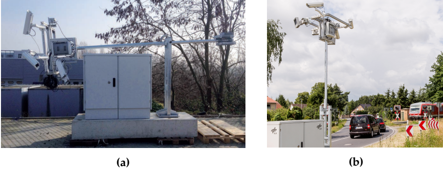
Fig. 2.9: The National Aeronautics and Space Research Center of the Federal Republic of Germany (DLR) has developed the Test field AIM (Application Platform for Intelligent Mobility) which is seen in (a) transportation mode and (b) operation mode. Image source: [16].
