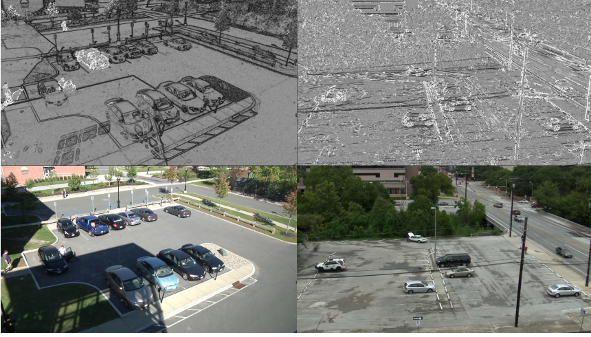
Fig. H.4: Two examples of the BGGRAD algorithm after running on videos from the VIRAT dataset. At the bottom are the RGB inputs, and above them are the corresponding foreground probability maps. On the right, is an example of what the output looks like when the algorithm runs on a shaky video, where all edges appears as foreground.
