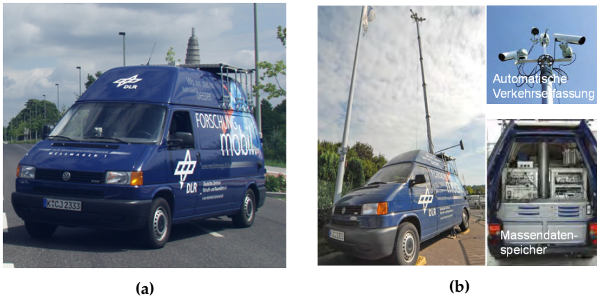
Fig. 2.8: The National Aeronautics and Space Research Center of the Federal Republic of Germany (DLR) has developed the Urban Traffic Research CAR. In (a) The UTRaCAR is seen with the telescopic mast retracted. (b) The DLR UTRaCar with the telescopic mast extracted. Image source: [15].
