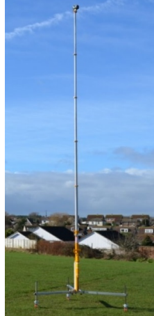
Fig. B.6: Clark QT Mast on tripod [15].
