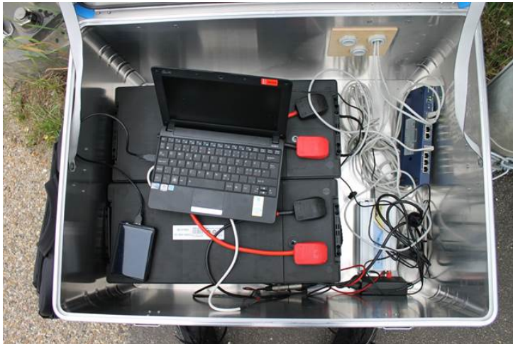
Fig. A.2: The Eurobox 40705 containing two batteries, a 220 V power converter, a PoE switch, and a netbook. The third battery is added by rotating the existing batteries 90 degrees.
