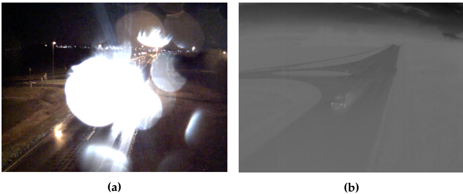
Fig. 2.2: Data collection at 02:00 in the night using two modalities. The (a) RGB camera has many problems in this lighting conditions, whereas the (b) thermal camera only senses the temperature making it more usable in large-scale studies. Image source: [1].
