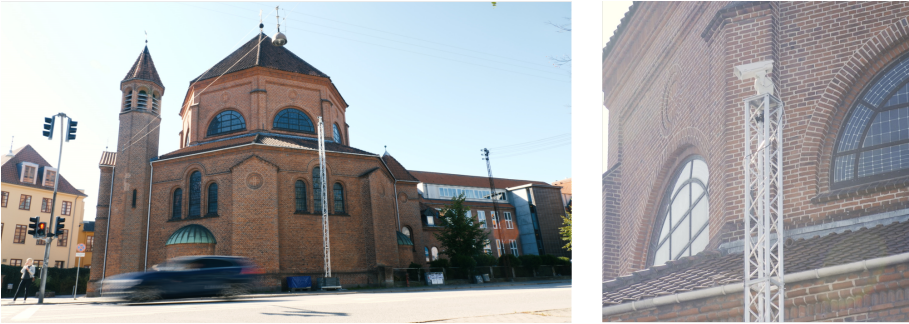
Fig. B.15: The portable pole deployed at traffic intersection. The pan-tilt motor with one RGB camera is installed on the top of the pole, which makes the RGB camera adjustable remotely.
