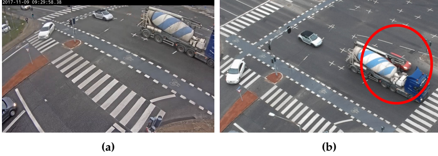
Fig. B.1: Objects can overlap each other in the camera-view as seen in (a) where the large cement truck clearly occludes the lane behind it. (b) clearly shows that a red car is in fact driving side-by-side of the cement truck.
