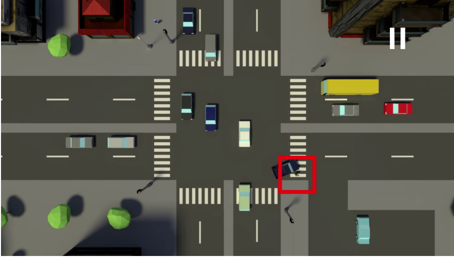
Fig. 2.4: Illustration of how drones provide a very nice overview of the traffic intersection, but due to regulation, the drone is restricted to a minimum height, causing some objects to be small and more difficult to detect in this view-angle, in this case, pedestrians (Marked with red square). Image source: [2].
