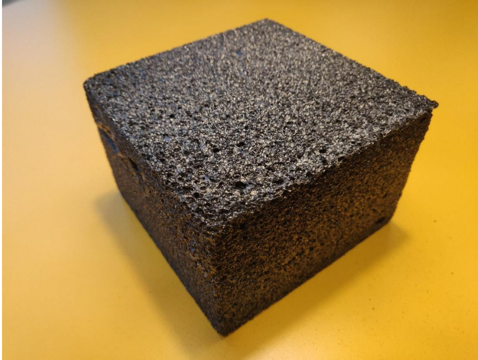
Figure 1: CleanTechBlock cellular glass sample.
