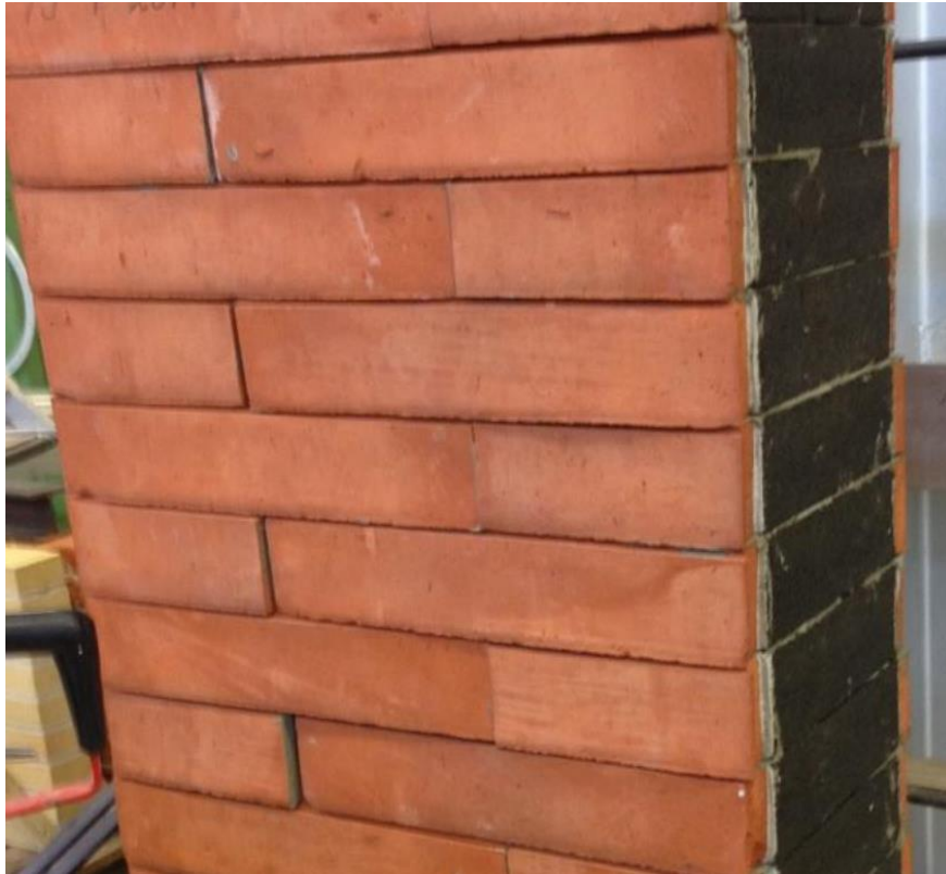
Figure 3: CleanTechBlock wall element: cellular glass blocks mounted in between 2 external layers of brick masonry [1].
