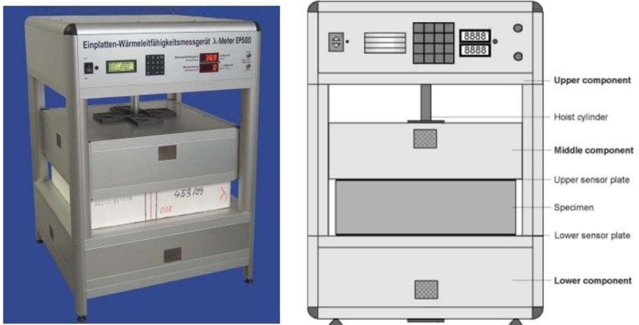
Figure 5: Guarded Hot Plate Apparatus EP500.
