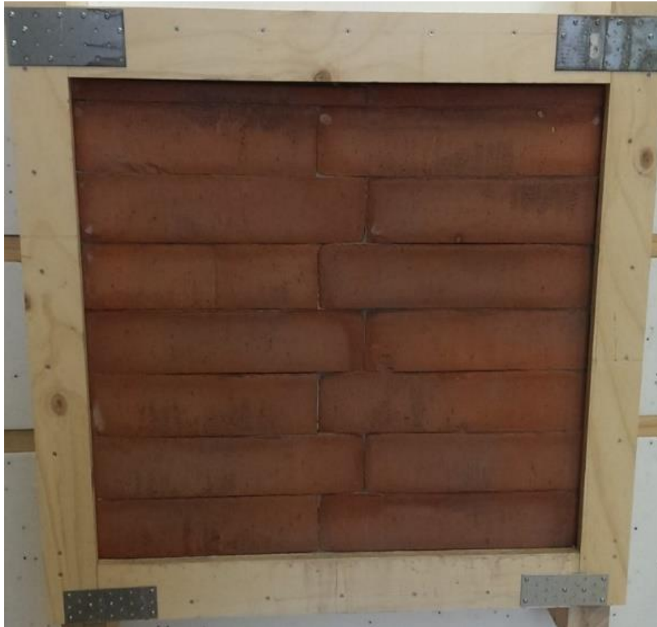
Figure 2: CleanTechBlock wall element mounted on insulation frame for Guarded Hot Box test.
