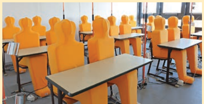
Fig. 8 Interior of the test-bed facility at Fraunhofer IBP Holzkirchen with dummies that emit both heat and CO 2 . Source: Fraunhofer IBP
