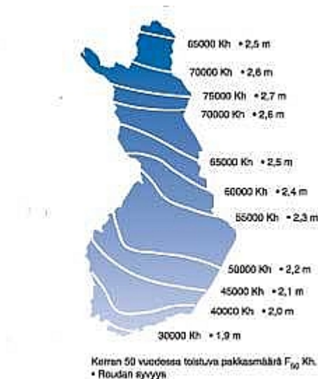
Figure 40: The dimensioning frost free depths for unheated buildings in Finland. Also dimensioning heating degree hours [Kh] are given. F_{50} gives the probability for these degree hours once in 50 years. [15]
