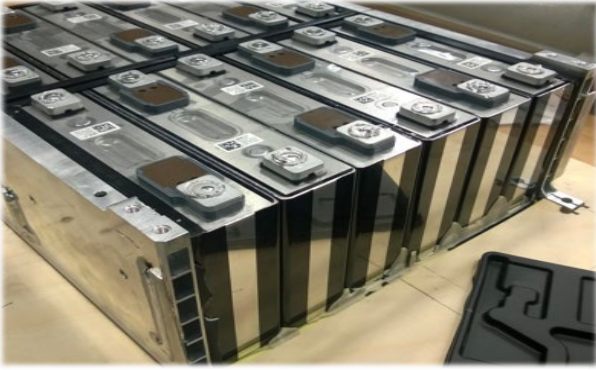
Fig. 1: BMWi3 battery module being disassembled.
