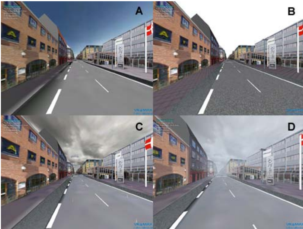
Figure 11.1: The same realtime 3D scene visualised with a) sunshine, blue sky and shadows, b) neutral, c) dark, rainy weather and d) fog.
