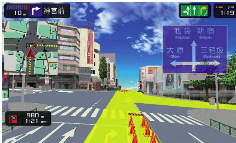
Figure 1.10: Sony's 3D map navigation technology for cars. The 3D mapping interface shows actual buildings, and knows street addresses, enabling it to identify destination addresses.
