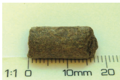
Photo 1: View of the design of typical DantoPlug Super pellet with 8 mm diameter.
