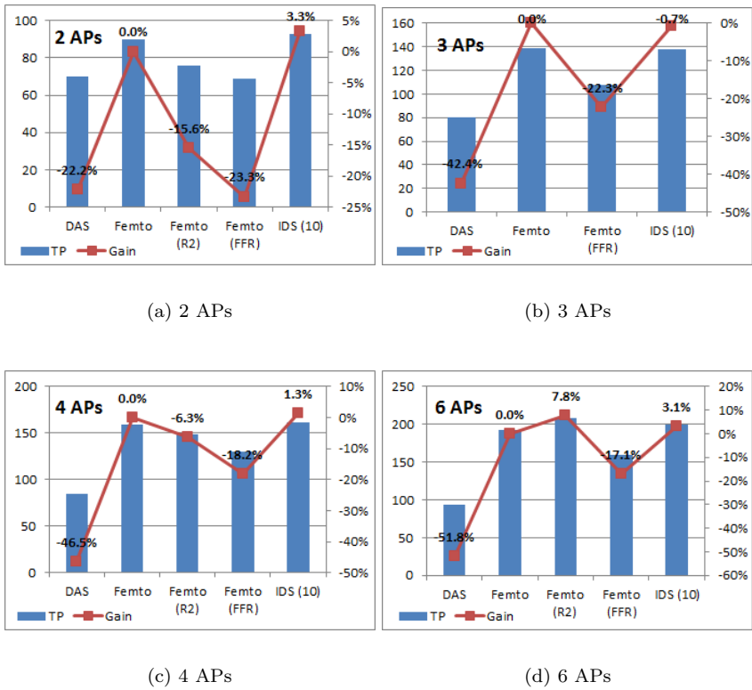
Figure C.2: Comparison of overall system throughput of different systems according to different numbers of APs.
