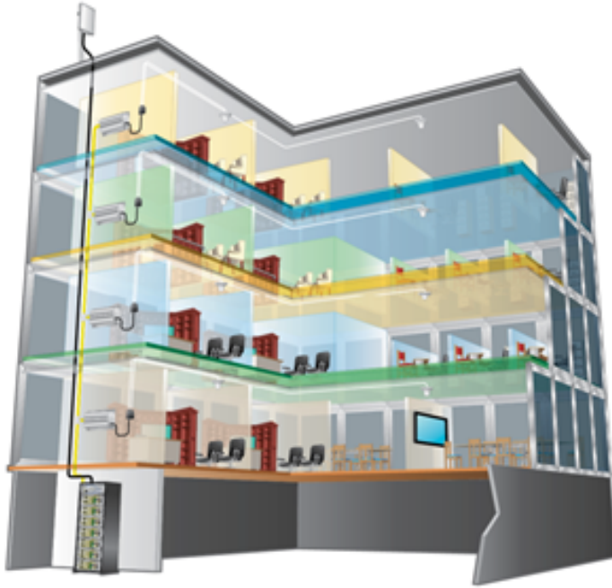
Figure 2.2: An example of the DAS deployed indoor.
