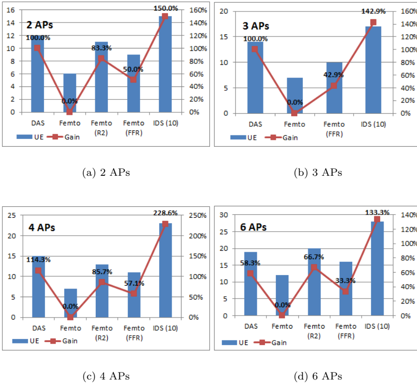
Figure 3.4: Comparison of maximum simultaneously supportable number of QoS users of different systems according to different number of APs.
