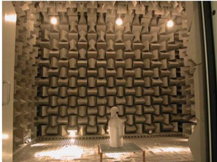
Figure 2.3: Inside the small anechoic chamber at Aalborg University
