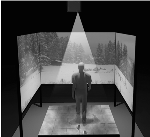
Fig. 8. Depiction of the multimodal VE developed by Law et al. (2008), incorporating a CAVE-like visual VE with an auditory and haptic floor display based on the Eco Tile. Footstep events in an immersive snowy landscape are accompanied by visual, auditory, and haptic feedback.
