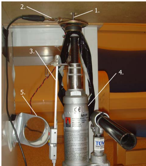
Fig. 3 The setup. 1 The stainless steel bolt attached to the pc speaker, 2 a cord connecting an ohm meter to the bolt, 3 a digital ruler, 4 the jack, 5 a mirror used for reading the digital ruler while operating the setup
