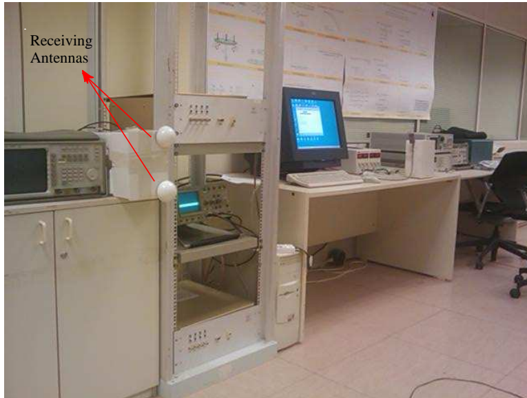
Figure 5.5: A setup showing the two receiving antennas (the two white hemispheres on the left side of the figure).
