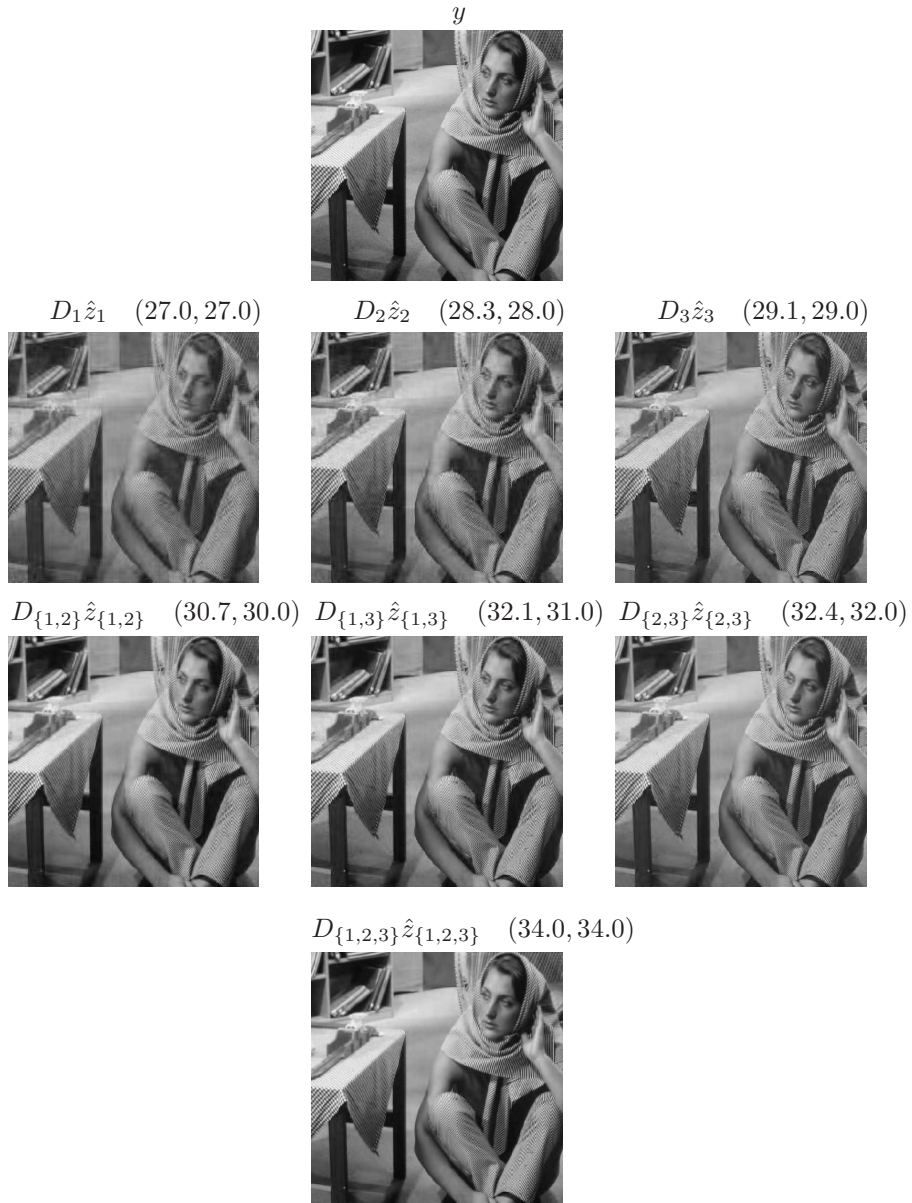
Fig. E.8: Encoding the image Barbara (Grayscale, 512 \times 512 ). As dictionaries we use D_{\{1\}}^{-1} : a 2-dimensional orthogonal Symlet8 DWT with 7 levels, D_{\{2\}}^{-1} : a 2-dimensional orthogonal Symlet16 DWT with 7 levels, and D_{\{3\}}^{-1} : a 2-dimensional biorthogonal CDF 9/7 DWT with 7 levels. We have \lambda_1 = 1.5, \lambda_2 = 1.4 and \lambda_3 = 1.0 . The distortion requirements and actual distortions are given above the individual images using the notation (\text{PSNR}(\|D_\ell \hat{z}_\ell - y\|_2), \text{PSNR}(\delta_\ell)) . The resulting rates are respectively R(\hat{z}_1) = 0.32, R(\hat{z}_2) = 0.52, R(\hat{z}_3) = 0.58 such that R(\hat{z}) = 1.42 .
