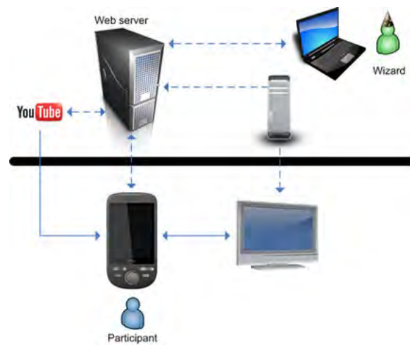
Fig. 1. Technical setup of the content transfer experiment
