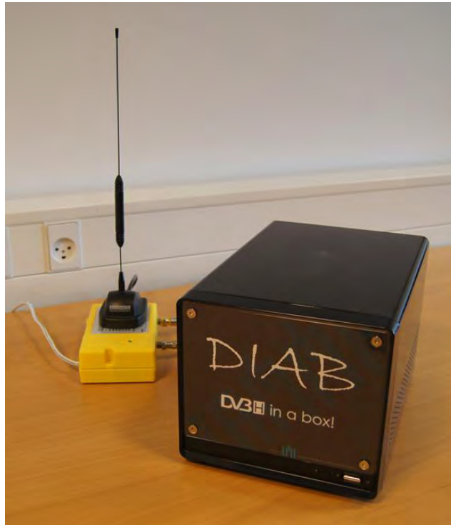
Figure 6.6: Elements of the DIAB transportable DVB-H testbed.
