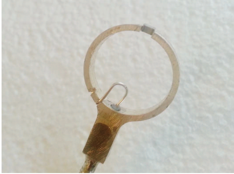
Fig. D.19: Antenna structure minimizing the use of tin.
