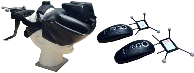
Figure 4.2: The devices used in all experiments. (Left) The nVisor SX111 HMD mounted on a styrofoam head. The HMD features 1280 \times 1024 pixels for each eye, and a total horizontal FoV of 102^\circ . However, the HMD only features stereoscopic overlap in the central 66% of the total FoV. (Right) The two wireless presentation mice used in the experiment. The mice each feature the usual 3 mouse buttons and a scroll wheel.
