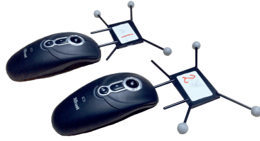
Figure C.1: The mice used in the experiment. Each mouse is fitted with reflective markers to make it detectable by an infrared camera system. The mice are equipped with the three usual mouse buttons as well as a scroll wheel.
