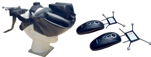
Figure B.5: The HMD and mice used in the experiment. The HMD and both mice are fitted with infrared reflective markers to be identifiable by the OptiTrack system.
