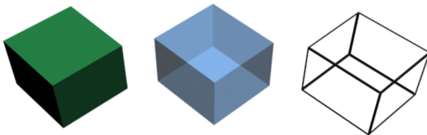
Figure 3.3: The same rectangular box rendered in three different ways. (Left) Rendered using the simple Blinn-Phong reflection model (Middle) A transparent version of the box, where both the external and internal faces are visible. (Right) Rendered using 2-sided wireframe mode. The wireframe version reveals that the box is, indeed, isomorphic to the box graph.
