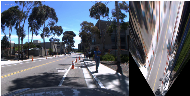
Fig. F.2: Native camera view on the left and top-down view generated via IPM on the right.
