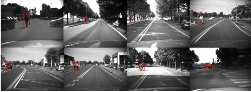
Fig. D.15: Examples of detection on a prototype platform. People in different poses are detected, including cyclists or people walking close a tree often hard to detect. A missed detection is shown in the last figure due to overexposure of the pedestrian.
