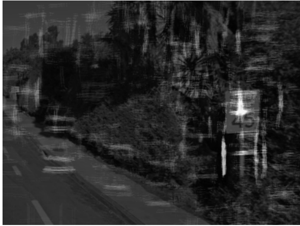
Fig. A.11: Votes from a radial symmetry system superimposed to the original image. The brightest spot coincides with the center of the sign. This image is from a system developed in conjunction with this paper and is a radial symmetry voting algorithm extended to work for rectangles
