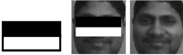
Fig. 3.2: Haar-like feature overlaid on a face. The value of this feature is computed by summing the values of the pixels under the black rectangle and subtracting the sum of the pixels under the white rectangle. Image credit: Soumyanilsc / CC-BY-SA-4.0 / http://enwp.org?curid=37353395
