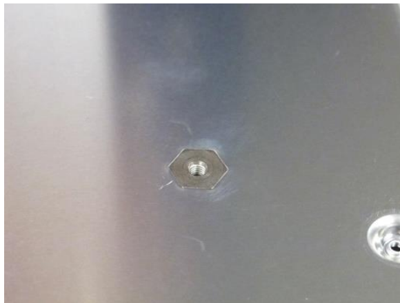
Picture 11-12: Screw thread made of iron or stainless steel embedded in aluminium.
