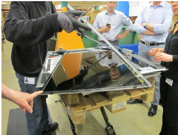
Picture 11-9: Glass front of B&O's television; this cannot be recycled.
