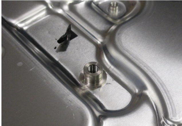
Picture 11-13: Screw thread made of iron or stainless steel embedded in aluminium.
