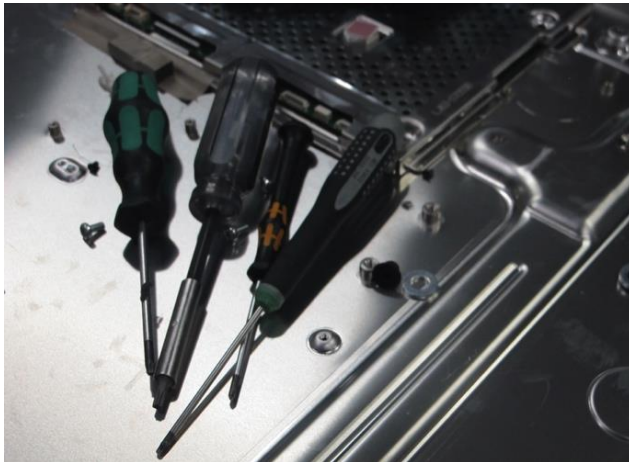
Picture 11-2: A picture of some of the different screwdrivers used to separate the television.
