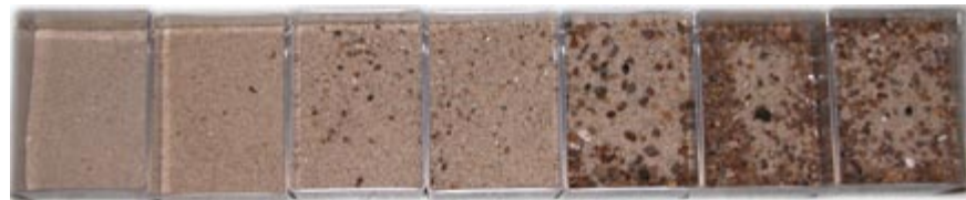
Figure 5. Illustration of the wide material composition, grain size and sorting span of the natural coastal sand calibration set. Note significant differences especially regarding particle size, the objective of the present study.
