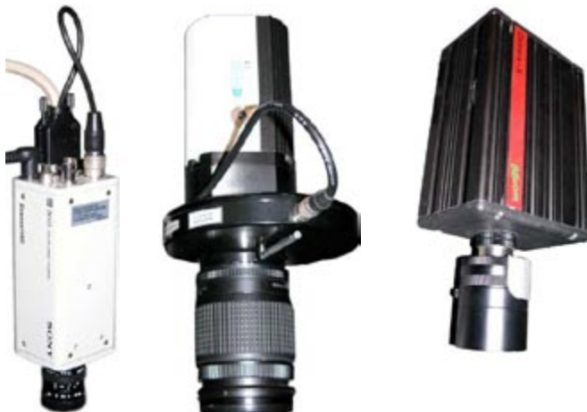
Figure 24. Examples of different camera types: Left: Sony 3-CCD camera. Centre: QImaging b/w camera with color wheel. Right: Camera X line-scan camera (BBcom).
