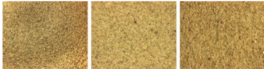
Figure 9. Photographs of the same sand sample, illustrating contrast differences resulting from the three alternative illumination sources. Photos (left to right) were obtained using the darkfield ringlight, ringlight and the LHS-500 lamp, respectively.
