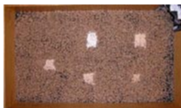
Fig. 14. Box after random sample extraction by the “spoon method”.
