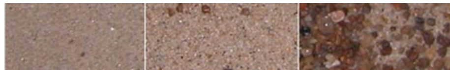
Figure 6. Close-ups showing extreme span in average particle size as realized in the master data set, as well as large differences w.r.t. particle size contrast (sorting). Images are to identical scale.
