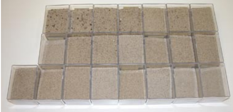
Figure 14. The combined (calibration, test) data set for the final third series (2 x 11 samples). Top left: highest D_{50} through lower right: lowest D_{50} . Every second sample in this lineup was selected alternatively for the training and the test set respectively.
