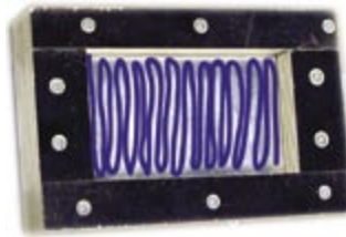
Figure 23. Bed-blending technique as used in this study. Whenever this technique is used, the material should become as evenly spread out as physically possible compared to when the material is poured into the sample container in one single pouring operation - which is a sure way of introducing maximum flow - and other segregation effects.
