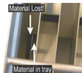
Fig. 5. Unwanted design error for the animal feed riffle splitter. If the tray is placed wrongly, as is very easy, almost half the material hitting the most peripheral chutes is lost.
