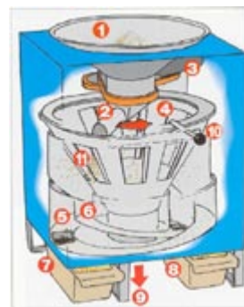
Fig. 10. Vario Divider. 1: hopper, 2: revolving feeder, 3: motor, 4: chute closer, 5 and 6: sample outlets, 7 and 8: samples, 9: left-over material, 10: chute opening handle and, 11: chute [19].
