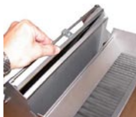
Fig. 9. The feeding tray opens “automatically” when tipped and gently pressed against the chutes. This takes place exactly at the center longitudinal axis. The small pin is inserted for controlling the width of the opening.
