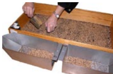
Fig. 13. Extraction of sample using the spoon method.
