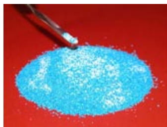
Fig. 35. Grab sampling—the world's worst mass reduction/sampling method! If the lot material is heterogeneous and/or segregated (which is most often the case), grab sampling is the simplest and fastest way to get heavily biased samples . A miniature riffle splitter can easily be used instead—adding only seconds to the total preparation time, but several orders-of-magnitude to the representativeness. Grab sampling is to be totally avoided!
