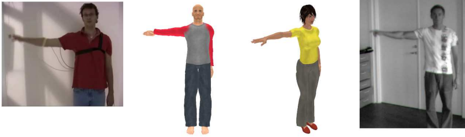
Figure 2.6: An illustration of the different types of data used in the system. From left to right: 1) 3D tracker data is acquired from magnetic trackers mounted on persons who perform the five actions. 2) The tracker data is animated in Poser from a fronto-parallel view. 3) The tracker data can be animated from any view point with different clothings and models. 4) After training the primitives on semi-sythetic data we recognize actions in real video.
