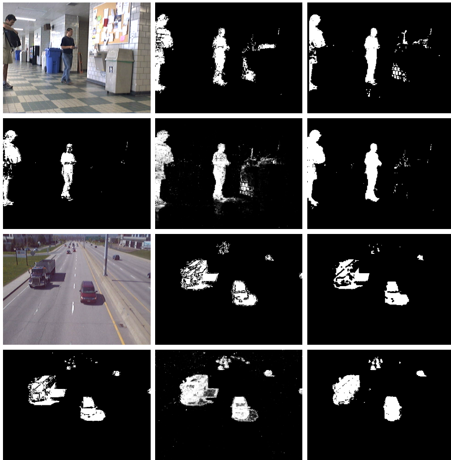
Figure 7.12: Original images from the HallwayI and HighwayIII sequences, and foreground results after shadow removal using the Huerta et al. approach [7], the Kim et al. approach [10], the Zivkovic et al. approach [24] using a shadow detector [17], the Martel et al. approach [12] and our approach, respectively (read row-wise).
