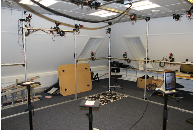
Fig. D.5: The lab setup for the second experiment. The iPad is placed on one of three platforms, all facing one corner of the room, in which the trackable marker is placed. In this example, the iPad is placed on platform #1. During the actual experiment it is moved between the platforms in random order.
