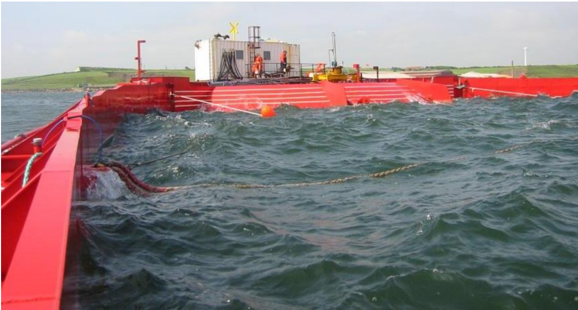
Figure 8: Illustration of a Phase 3 WEC prototype, the Wave Dragon scale 1:4.5 being tested in the benign site of Nissum Bredning [22].
