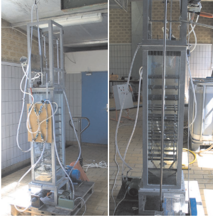
Figure 4.55 Pictures of the settling column as installed on Aalborg East WWTP in 2004.
