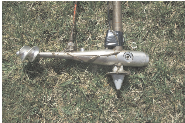
Figure 5.39 OTT impeller used for the measurements of time-averaged flow velocities. From: (Kunnerup et al. , 2002).
