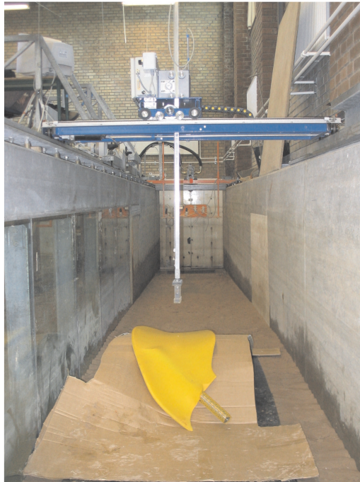
Figure 4.30 Experimental set up for measuring the geometry of the propeller blade.
