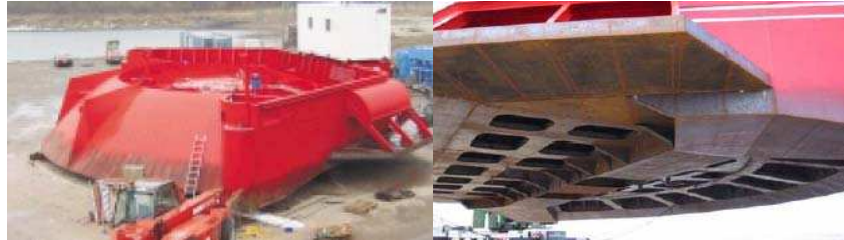
Fig. 1: The platform at the dockside in 2003 before being launched. On the right the open air compartments used for buoyancy regulation can be seen.
