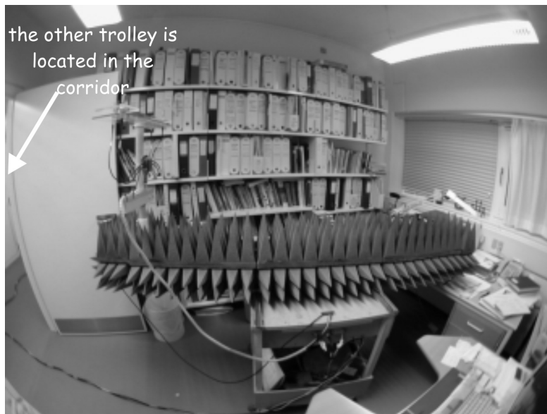
Figure 3.20: Second example of a MIMO radio channel measurements, fb7b2. The dragon is positioned in the middle of the room. Notice the space limitations to fit the dragon inside the office. The other trolley with all the RF equipment was in the corridor as illustrated in Figure 3.1.
