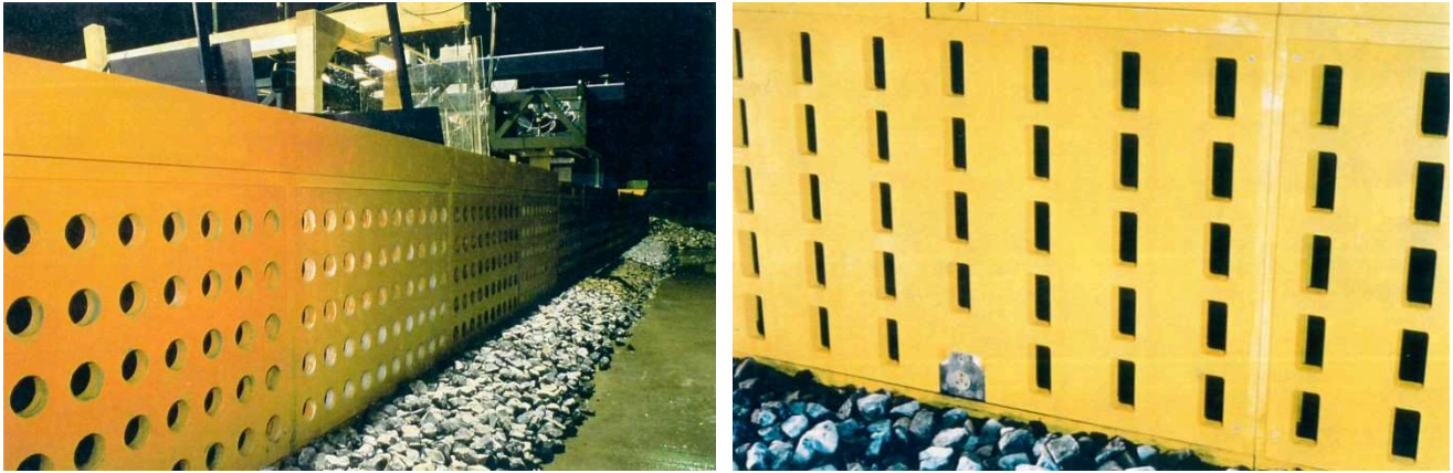
Fig. 7. Photos of the two types of perforated caissons tested in 3D (from Franco C. 1996).
