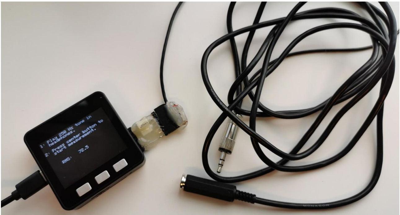
Figure 4.2 Calibration box designed for calibration and level adjustment of the headphones used with the system
