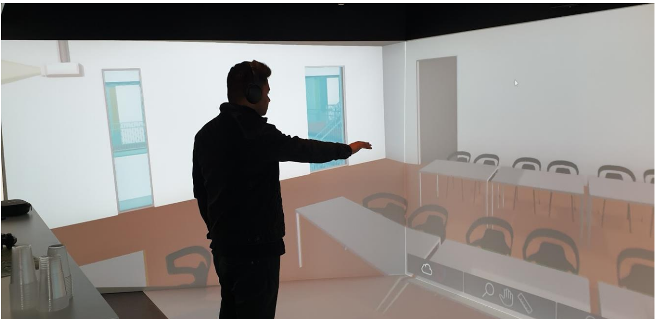
Figure 4.4 CAVE setup: Test-persons navigate sensors, whilst listening to the room using over-ear-headphones.
