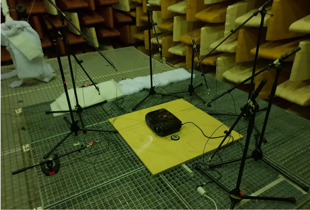
Figure 2.4 Recording sound of a projector in the anechoic room
