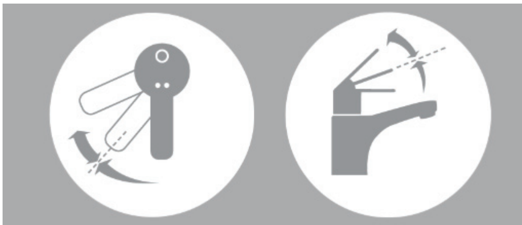
Figure 3.10: Principle for water saving mixer fixtures.
