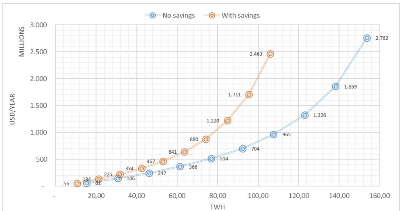
Figure 15. District heating investment costs in USD/year in relation to heat demand for scenarios without and with savings
