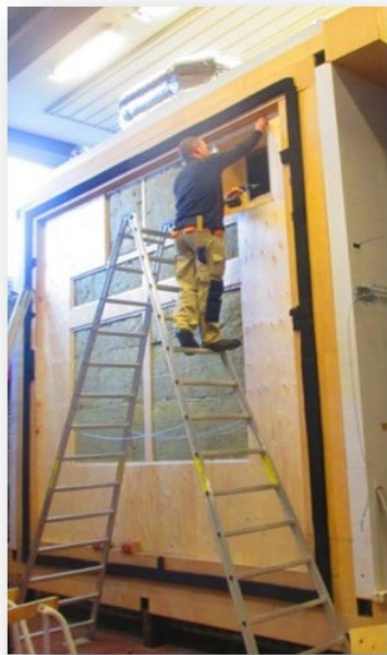
Figure 4: The Big Guarded Hot Box setup at Aalborg University, Department of Civil Engineering.
