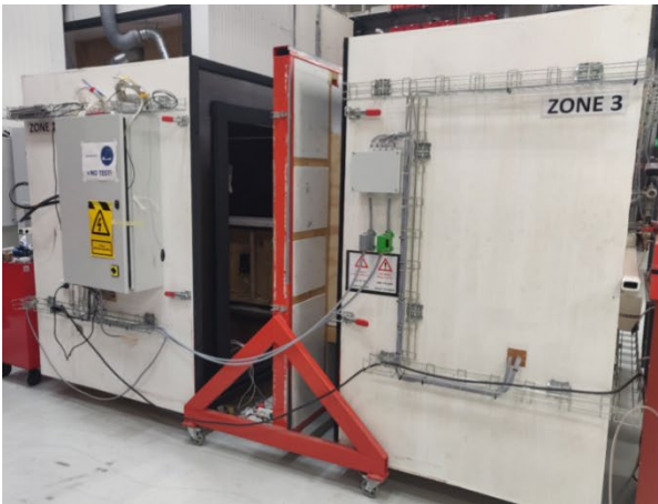
Figure 3: The Guarded Hot Box setup at Aalborg University, Department of Civil Engineering.
