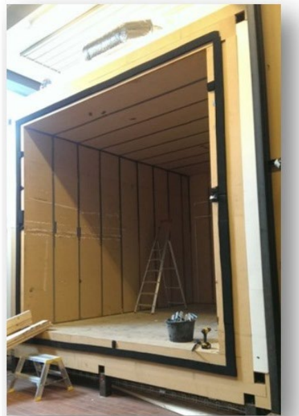
Figure 4: The Big Guarded Hot Box setup at Aalborg University, Department of Civil Engineering.
