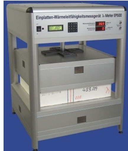
Figure 2: The Laser Flash Analysis Apparatus LFA 447 from Netzsch Gerätebau GmbH [5] (left); the Guarded Hot Plate Apparatus EP500 from Lambda-Messtechnik GmbH Dresden [6] (right).
