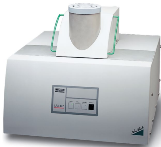
Figure 2: The Laser Flash Analysis Apparatus LFA 447 from Netzsch Gerätebau GmbH [5] (left); the Guarded Hot Plate Apparatus EP500 from Lambda-Messtechnik GmbH Dresden [6] (right).
